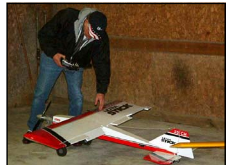
Bob King displays his Hangar 9 Ultra-Stik, with power provided by a Moki 1.80 and a Bolly 18x10 prop.
