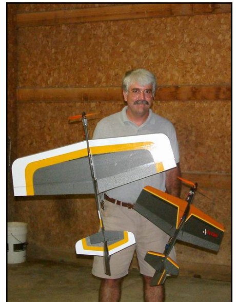
Karl Laun shows his electric Tridents in both the 36" and 24" versions. The Tridents are capable 3D parkflyers made from foam sheet.
