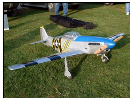
SIRS Field, October 11, 2003 — (Left) Chris Cochran assembles his Giant Scale Planes P-51 for its maiden flight. (center) The assembled model (right) The first flights were flown successfully, but ended in dead-stick landings. Chris' plan has a wingspan of 100" and weighs 27.75 pounds. It's powered by a 3W75 motor and features Robart retracts and scale wheels.
