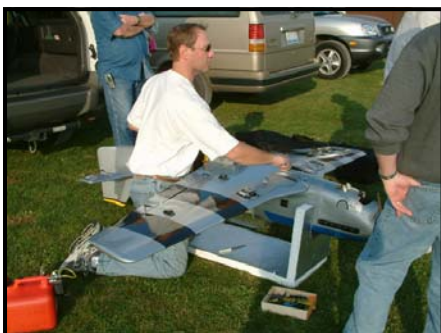
SIRS Field, October 11, 2003 — (Left) Chris Cochran assembles his Giant Scale Planes P-51 for its maiden flight. (center) The assembled model (right) The first flights were flown successfully, but ended in dead-stick landings. Chris' plan has a wingspan of 100" and weighs 27.75 pounds. It's powered by a 3W75 motor and features Robart retracts and scale wheels.
