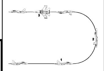
This comprises an ascending half-loop followed by a half-roll, resulting in level flight in the exact opposite direction at a higher altitude.
